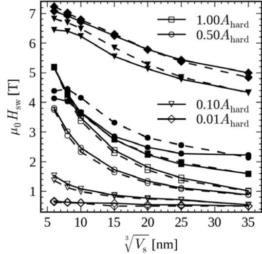
Fig. 3.  $\alpha\text{-Fe}$  cubes (solid line) and spheres (dashed line) enclosed by a 1 nm interlayer in a  $\text{Nd}_2\text{Fe}_{14}\text{B}$  spherical matrix. The interlayer exchange constant  $A_i = fA_{hard}$  is reduced to decouple inclusion and shell. Open markers refer to the soft phase reversal field and filled markers to the hard phase switching field.
