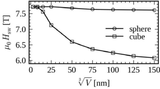
Fig. 1. Switching field of  $\text{Nd}_2\text{Fe}_{14}\text{B}$  cubes and spheres with volume  $V$ .
