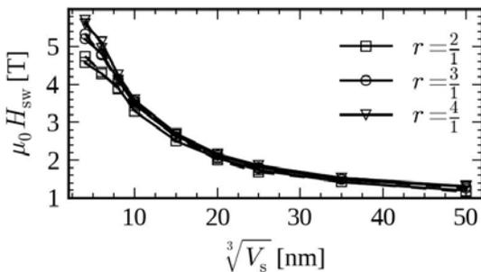
Fig. 2. Switching field of  $\alpha\text{-Fe}$  cubes (solid line) and spheres (dashed line) with equal volume  $V_s$  in a  $\text{Nd}_2\text{Fe}_{14}\text{B}$  spherical shell.  $r$  denotes the ratio of hard to soft magnetic volume.
