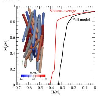
Figure 4: The computed reversal curve for the full model rod arrangement shows a 20% reduction in coercivity compared to the isolated volume-averaged results, due to magnetostatic interactions. Inset: visualization of the packed rods model.
