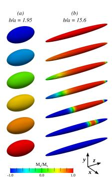
Figure 2: Visualizations of the computed magnetization data during reversal of soft prolate spheroids for aspect ratios (a) 1.95 and (b) 15.6, showing the different reversal modes.
