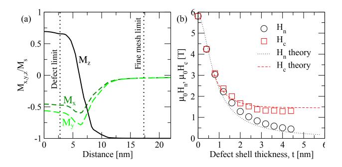
FIG. 3. (a) Plot of the saddle-point  $M_x$ ,  $M_y$  and  $M_z$  magnetization components along a diagonal from the reversal corner towards the opposite corner of the cube. The data is taken from the saddle-point configuration of a nudged elastic band (NEB) simulation, which is the highest energy magnetization configuration in the energy-minimized reversal path. (b) A plot of  $\mu_0 H_n$  and  $\mu_0 H_c$ against defect thickness t, with Aharoni's 1D defect model for comparison.
