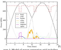
gure 1: Model of power generation grid including naive load model, coal, solar, wind and hydroelectric power sources. Various scenarios can be tested.
