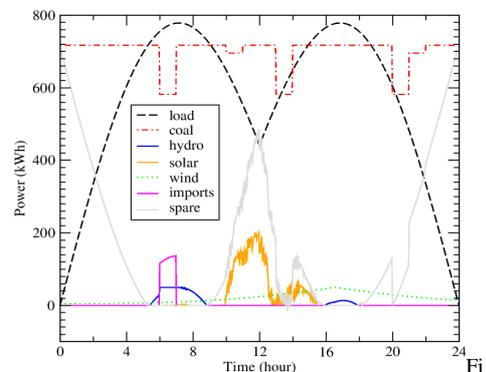
Figure 1: Model of power generation grid including naive load model, coal, solar, wind and hydroelectric power sources. Various scenarios can be tested.
